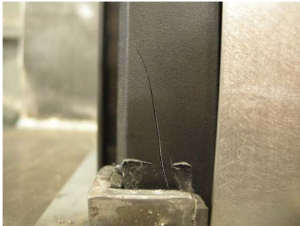
Crack in Front Plastic Control Panel Cover
