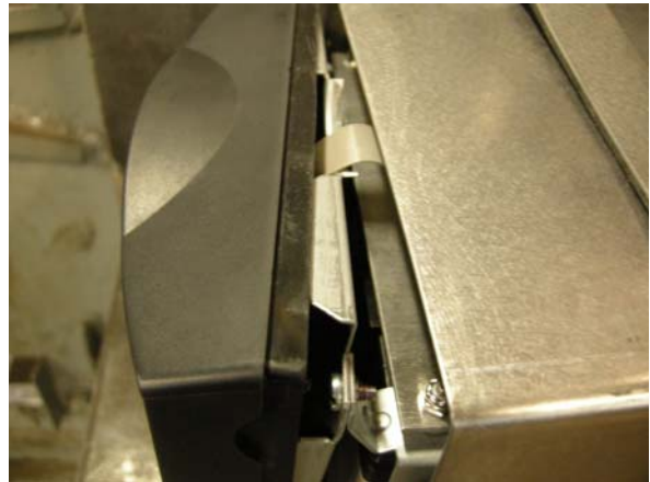
Damage to the Front Panel
