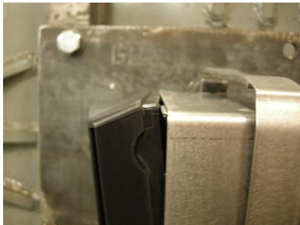
Damage to the Front of the Power Supply and Plate
