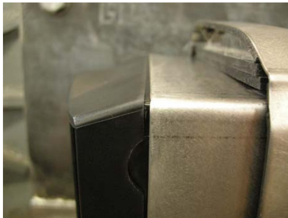
Front Plastic Control Panel Cover Pulled Away from Metal Frame
