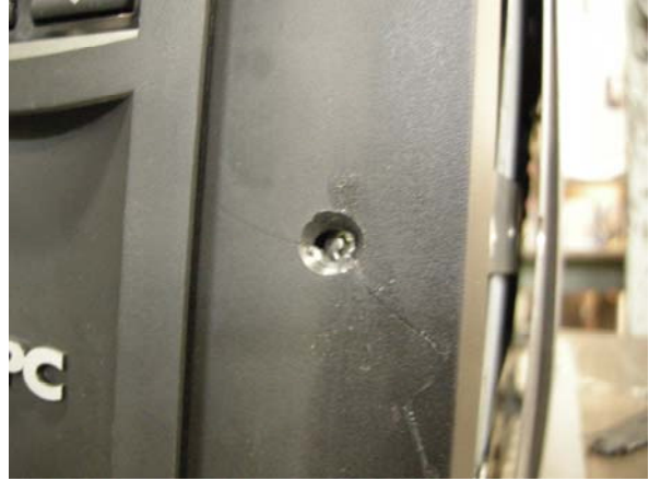
Front Panel, Source of Detached Screw
